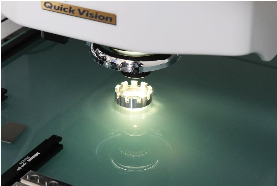
And with the Mitutoyo measuring machine, GFH kills three birds with one stone. Due to its measuring uncertainty of only  $0.25\ \mu\text{m}$ , the 3D CNC vision measuring machine is perfectly suited for the calibration or compensation of their own machines. Thus, it can measure circular-lasered test workpieces with an accuracy of up to one micrometre.
